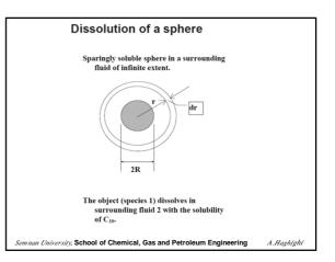
$$\begin{pmatrix} \text{Rate of} \\ \text{mass in} \end{pmatrix} - \begin{pmatrix} \text{Rate of} \\ \text{mass out} \end{pmatrix} + \begin{pmatrix} \text{Rate of mass} \\ \text{production} \end{pmatrix} = (\text{Accummulation})$$
